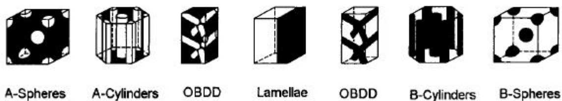
Figure 3.4: Different classes of structures in diblock-copolymers. According to the ratio between the degree of polymerisation of the A's and B's, N_A and N_B , the different classes form. For N_A \ll N_B spherical inclusions of A in a B-matrix are formed and they set up a body-centred cubic lattice. For larger value N_A , but still N_A < N_B , the A-domains have a cylindrical shape and they are arranged in a hexagonal lattice. Layered lattices form under essentially symmetrical conditions, i.e. N_A \approx N_B . Then, for N_A > N_B , the phases are inverted, and the A-blocks now constitute the matrix. The 'ordered bicontinuous double diamond' (OBDD) structures exist only in a narrow range of value N_A/N_B , between the regime of the cylindrical and lamellar structures.
