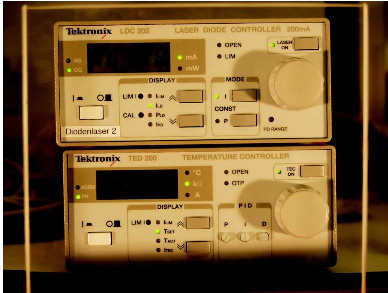
Figure 8: Current and temperature controller for diode laser. Settings should not be changed.
