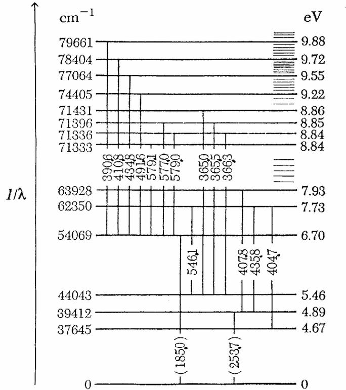
Figure 1: Level scheme of the neutral mercury atom.
