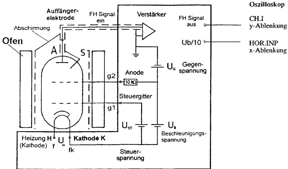
Figure 4: Circuit diagram for the Franck-Hertz tube.
