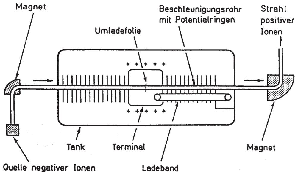
Figure 7: Principal Sketch of a Tandem Accelerator
