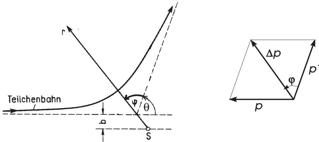
Figure 3: Kinematics of coulomb scattering off the scattering center S.
