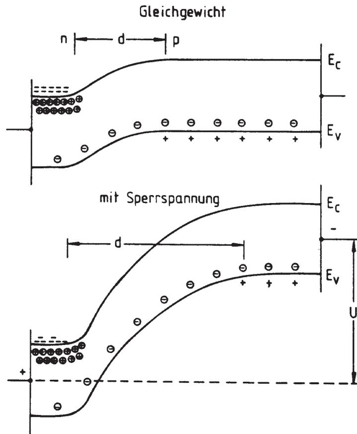
Figure 10: Band structure of an asymmetrical p-n transition;  $d$ : thickness of depletion layer,  $E_c$ : lower boundary of conduction band,  $E_v$ : upper boundary of valence band,  $U$ : reverse-bias voltage.
