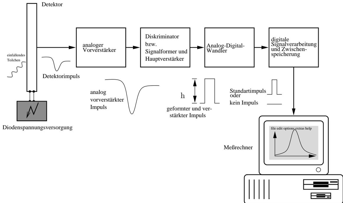
Figure 11: Schematic setup of the data acquisition of the experiment
